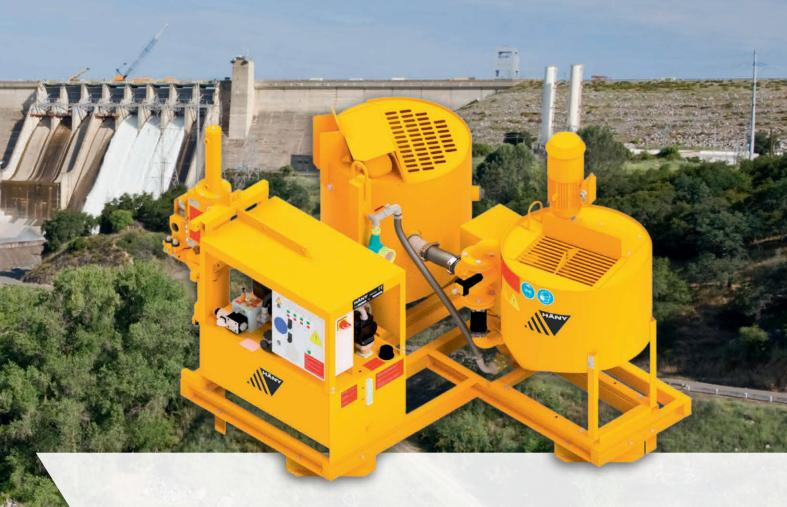
The compact grout plants consist of the proven, standard Häny components of a mixer, agitator, and grout pump. This setup is suitable for a wide range of applications such as anchoring, sleeve pipe, contact, and backfill grouting. For higher outputs and increased quality control, the plants are also available in semi-automated and fully automated versions.
